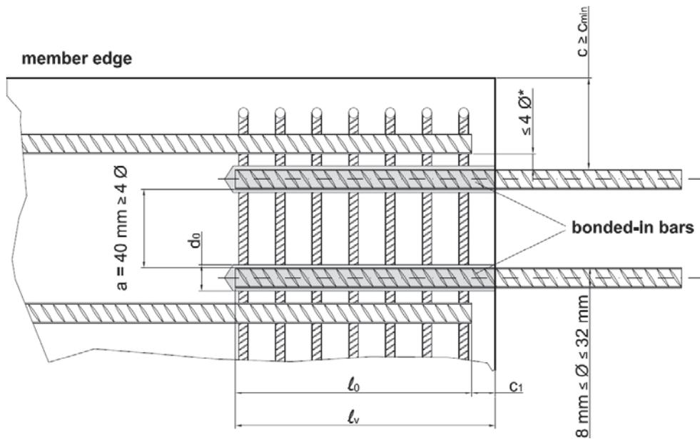
\* If the clear distance between overlapping rebars is greater than  $4 \cdot \emptyset$  the overlap length shall be enlarged by the difference between the clear distance and  $4 \cdot \emptyset$ .
