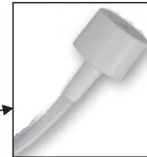
Insert the special mixer extension in the inner diameter of the injection plug up to reach the top of the plug
